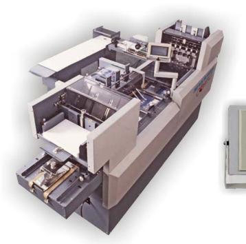
Cperator control of is through a touch screen. This enables station selection and output speed, error location and further run information.
